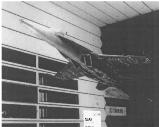
Fig. 2 F/A-18E force and moment model, 8% scale.
